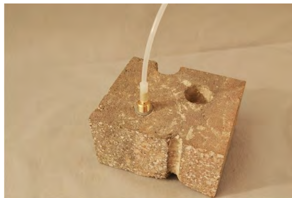
Figure 5. Vapor Pin™ sample connection.
